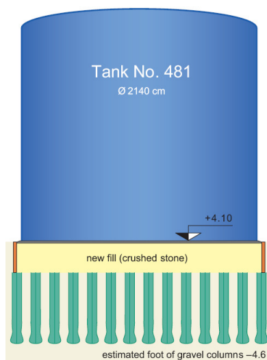
Pic. 6 - Tank with stone columns
