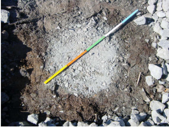
Pic. 3 - Cross-section of grouted stone column
