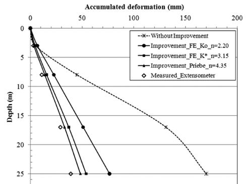
Figure 8. Accumulated compressibility results of field test.
