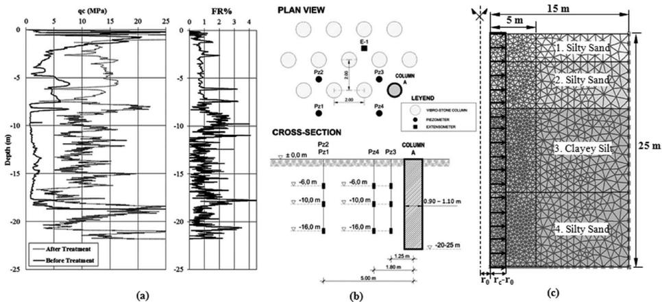
Figure 2. Field test characteristics, (a) cone penetration resistance after and before the treatment, (b) plan view and section of field test and (c) geometry of finite element modelling.
