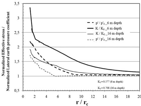
Figure 6. Distribution of effective mean stress and coefficient of lateral earth pressure.
