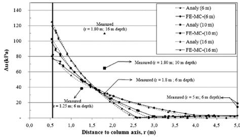
Figure 5. Estimation of excess pore pressures due to vibro-stone column installation.
