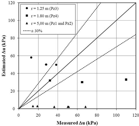
Figure 3. Predicted and measured peaks of excess pore pressures.
