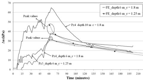
Figure 4. Measurements of excess pore pressure dissipation.
