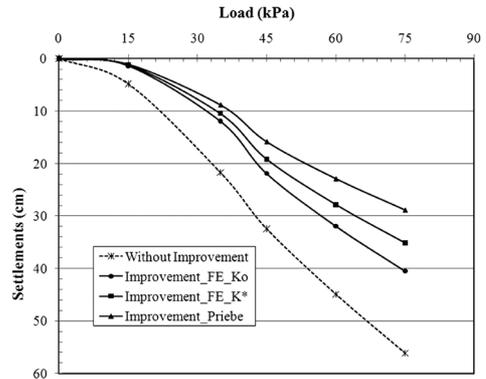
Figure 7. Load settlements results of field test.
