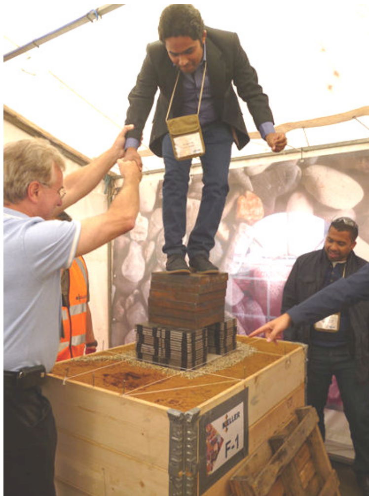
Figure 6. After the serviceability testing, the model is loaded to failure
